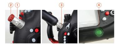
As long as the green LED is blinking, the vacuum inside the housing is stable. This indicates that the housing is properly closed and that it is safe to take it underwater. In case of a leak, the pressure inside the housing will increase. An increase of pressure of 40mbar will trigger the red LED and will produce beeps. If this situation occurs, check all the housing and port seals and start the vacuum procedure again.
