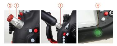
As long as the green LED is blinking, the vacuum inside the housing is stable. This indicates that the housing is properly closed and that it is safe to take it underwater. In case of a leak, the pressure inside the housing will increase. An increase of pressure of 40mbar will trigger the red LED and will produce beeps. If this situation occurs, check all the housing and port seals and start the vacuum procedure again.
