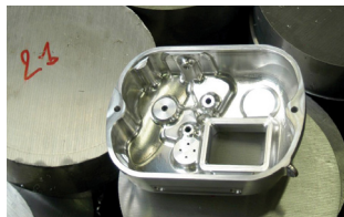
Your Hugyfot housing has been milled out of a solid block of seawater resistant aluminum.
