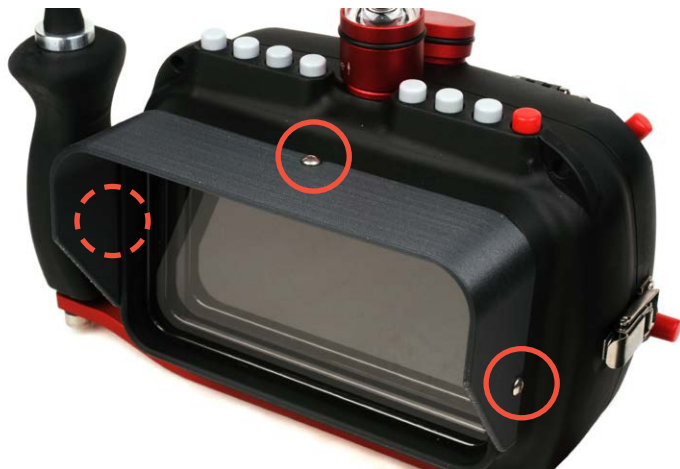
The sun hood of your Hugyfot Vision Xs housing is secured with three M3 screws (left, top, right).
