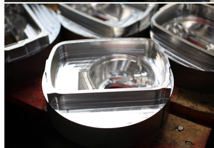
Your Hugyfot Vision Hero 5 housing is machined from a solid block of marine grade aluminum.
